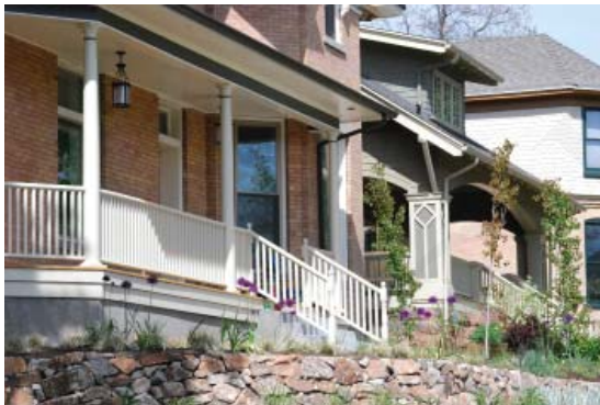
A coincidence of setbacks and common eaves height help to create an affinity between individual house scales and styles.
