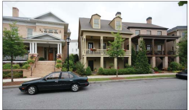
A variety of building forms, roof profiles and entrances share common heights with strong horizontal elements. Equally strong vertical features are evident in the columns, bays and dormer windows.
