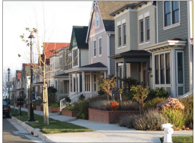
Several building designs and forms create variety and visual vitality, yet instill a strong vertical visual emphasis using facade or module width. Single story porches and projecting window bays sharing a common eaves height establish a rhythm.
